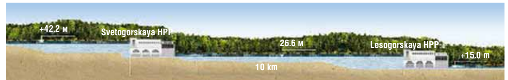
Fig. 39. Cascade operation scheme with Vuoksa HPP Cascade as an example
